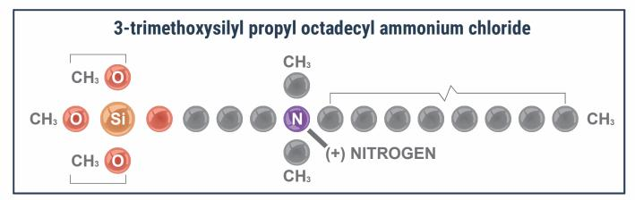
The silane base acts as an anchor, securing the antimicrobial to almost any hard surface or substrate.
